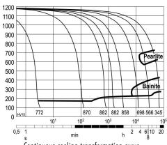
Continuous cooling transformation curve Hardening Temperature 1180°C
