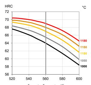
Tempering Temperature °C Hardness after hardening, quenching and tempering 3x1 hour
